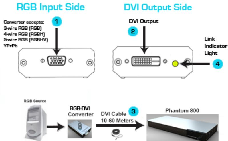
**FIGURE 9.** RGB-DVI Converter installation
