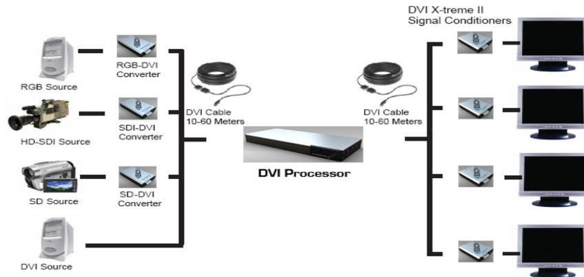
**FIGURE 1.** System diagram using DVI Converters
