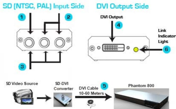
**FIGURE 7.** Phantom-Powered SD-DVI Converter installation
