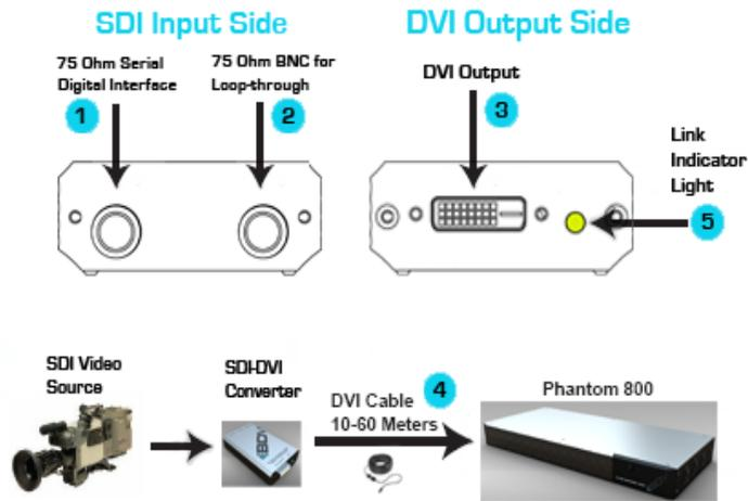
**FIGURE 8.** Phantom-powered SDI-DVI Converter installation
