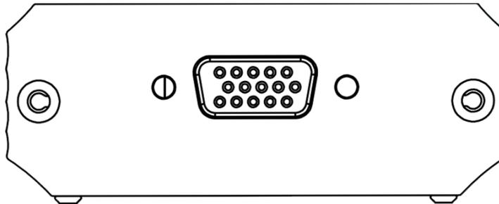
**FIGURE 4.** RGB/YUV input panel of the RGB-DVI Converter
