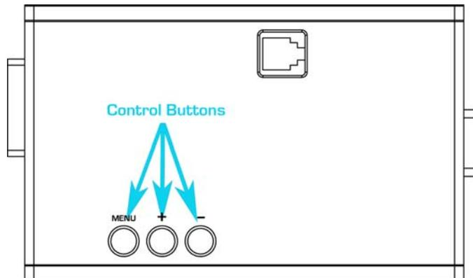
**FIGURE 10.** Control buttons on an externally-powered converter
