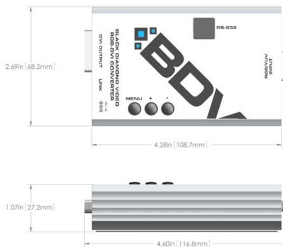
**FIGURE 2.** Externally-Powered RGB-DVI Converter dimensions (same for all BDV converters)
